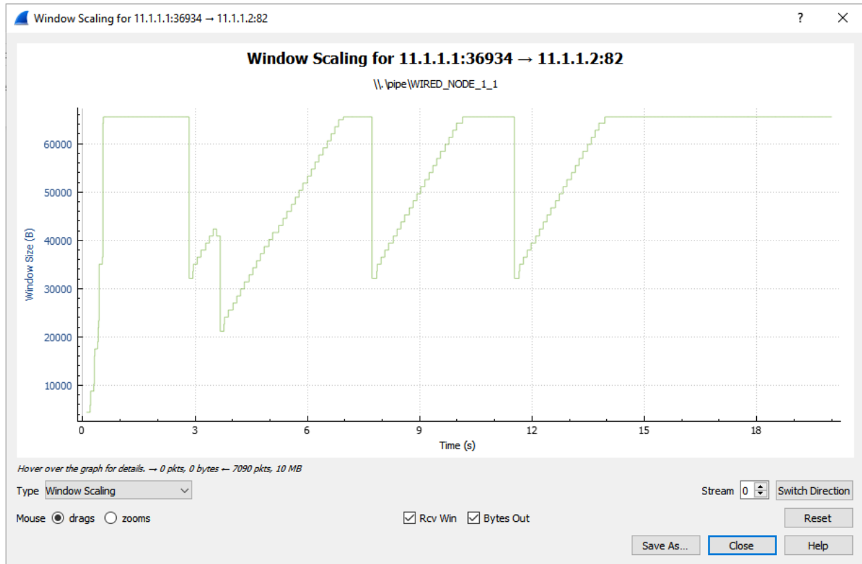
Figure 1-6: Congestion window evolution with TCP New Reno. We note that New Reno infers packet loss with timeout and triple duplicate acknowledgements, and updates the slow-start threshold ssthresh and congestion window cwnd as ssthresh = cwnd/2 and cwnd = ssthresh + 3MSS (in the event of triple duplicate acknowledgements).
