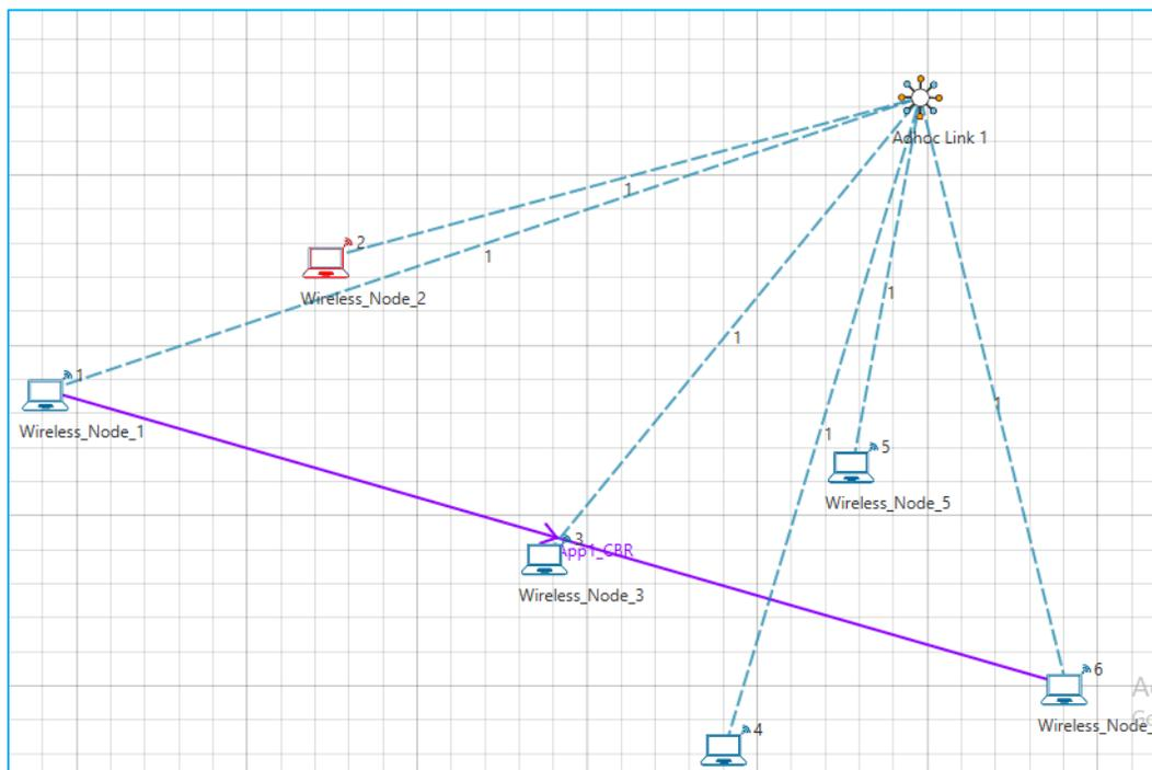
**Figure 1:** Created network topology with 5 Wireless nodes
