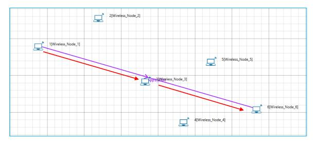
Flow of packets after node 2 is detected as malicious
