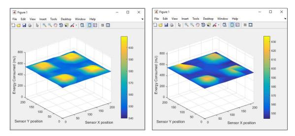
In the initial phase the plot resembles the previous one. However as the time passes, it can be observed that the power is consumed by all the sensors at approximately the same rate.
