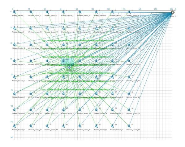
**20.** Run the Scenario. You will observe that as the simulation starts in NetSim, MATLAB gets initialized and graph associated with energy consumption in the sensor network is plotted during runtime.
