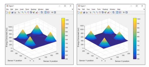
As it is seen from the plot, there are 4 peaks in the plot corresponding to higher energy consumption in the nodes in the center of the cluster, as they always become the cluster heads. This is because distance is used as a parameter for electing the cluster heads.
