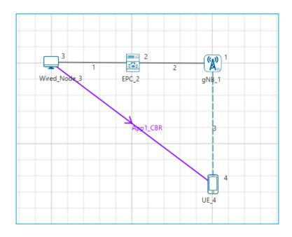
The network configuration has the initial distance between the gNB and UE as 50 meters with the gNB located at (1000,200) and UE located at (1000,250).
