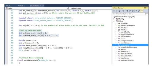
Right click on Solution in Solution Explorer and select rebuild solution.
