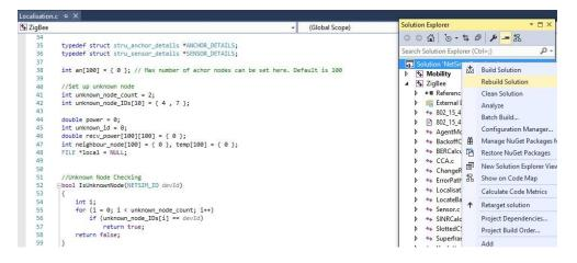
Upon rebuilding, libZigbee.dll and libMobility.dll will automatically get updated in NetSim binary folder. **Note:** Based on whether you are using NetSim 32 bit or 64 bit setup you can configure Visual studio to build 32 bit or 64 bit Dll files respectively as shown below:
