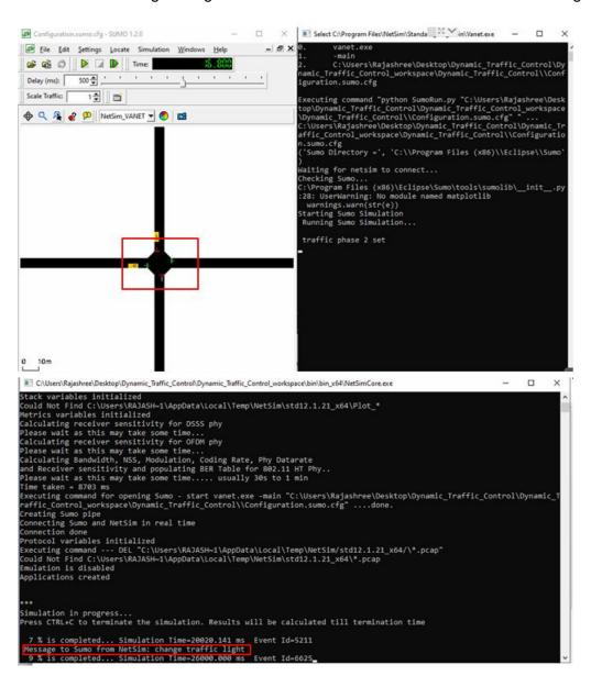
4. Traffic signal changes from phase 2 to phase 3 indicating that vehicles in the EW lane have to slow down due to the control message received by NetSim in the sumo console is shown below.
