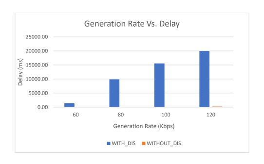
We can observe that the application throughput decreases in case of DIS flooding when compared with the usual simulations for various application traffic generation rates.
