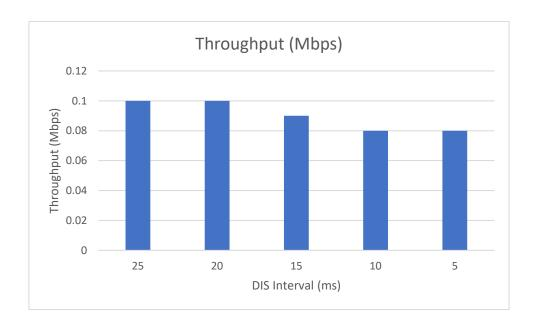
We can observe that the application throughput decreases as we decrease DIS Interval time. Upon decreasing the DIS interval, more DIS messages will be sent by the malicious nodes more frequently. Legitimate sensors spend more time in processing and responding to DIS messages than sending the data packets.
