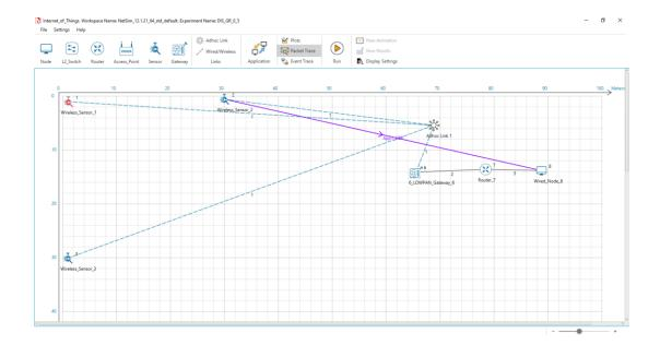
Source – Device id 2 Destination – Device id 8 Sinkhole (malicious node) – Device id 1
