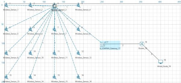
2. Configure traffic in the network by setting a few applications between some of the sensor nodes to the Wired Node using the Application Icon, as shown below:
