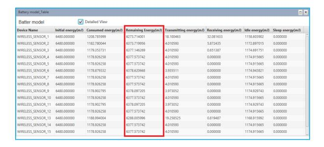
Now on comparing the custom IOT metrics we can observe that Energy Harvesting increases sensors' working capability. Simulations can be performed for different values of EH Fraction which may vary as per the efficiency of the Energy Harvesting unit.
