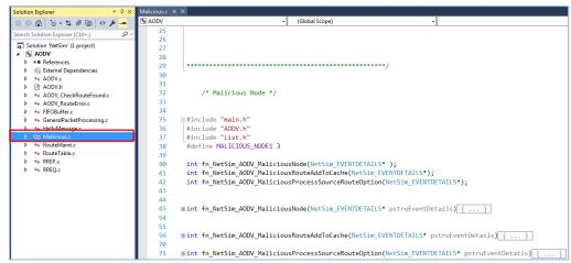
You can set any device as malicious and you can have more than one malicious node in a scenario. Device id's of malicious nodes can be set inside the <a href="mailto:fn\_NetSim\_AODV\_MaliciousNode">fn\_NetSim\_AODV\_MaliciousNode</a> () function.
