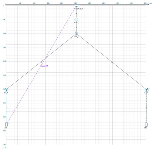
1. Simulate the scenario in Netsim and you will get two .csv files in bin folder of Netsim corresponding to each UE's involved in the simulation. Open any .csv file of the UE for which File Based Mobility was configured. You will observe the columns containing SNR measured by each ENB with respect to that particular UE.
