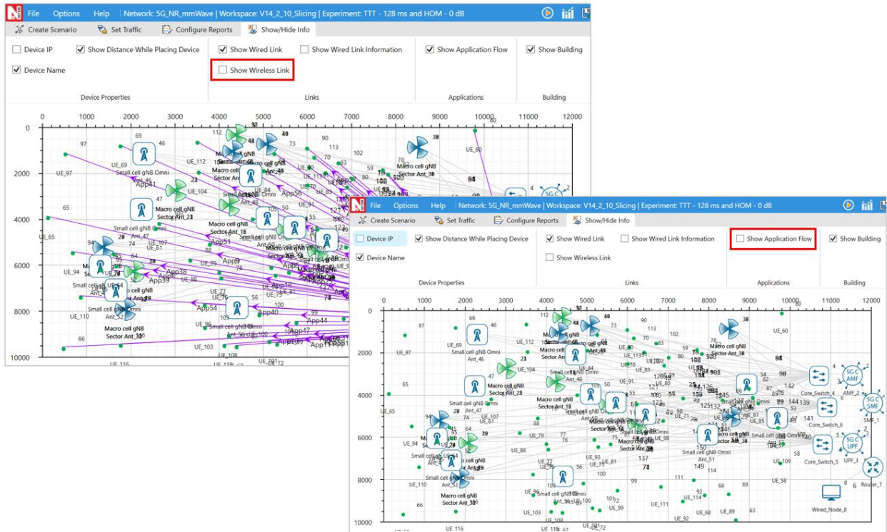
Figure 3-46: Disabling the wireless link and application flow from Show/ Hide Info tab
