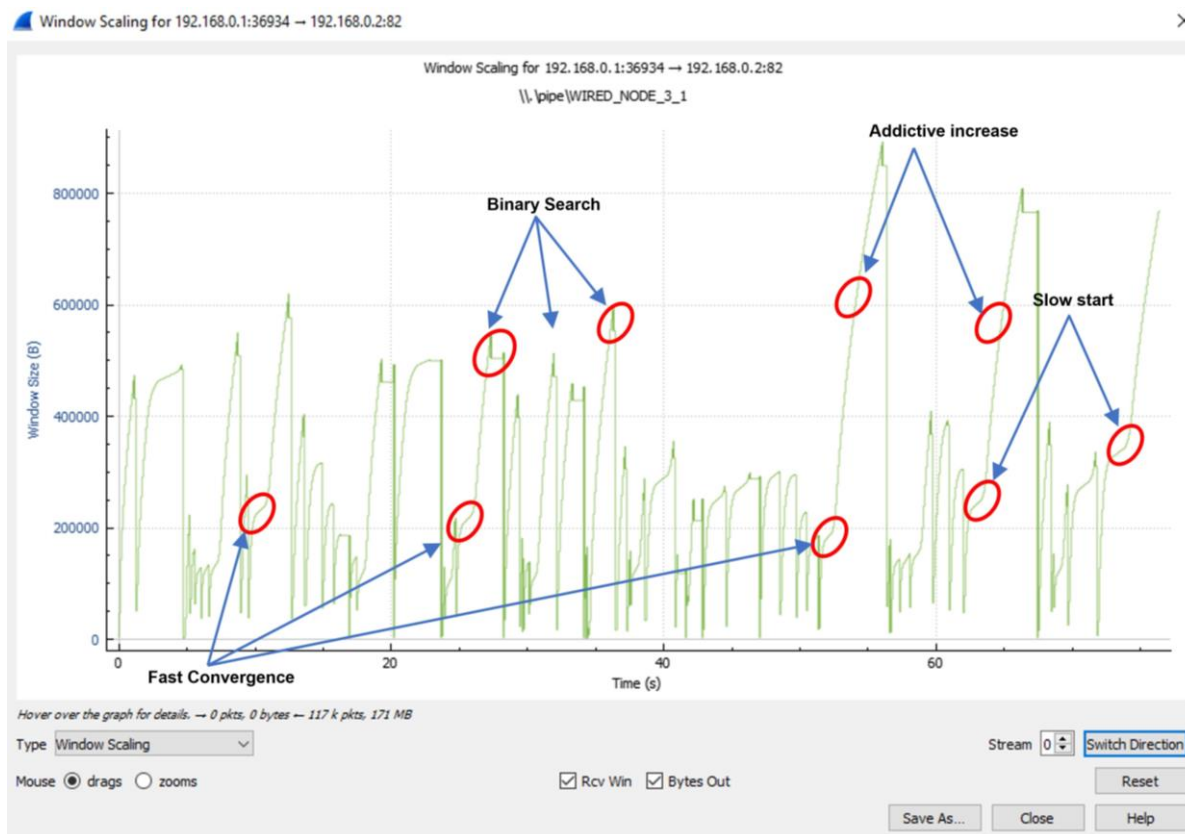
Figure 4-30: Plot of Window Scaling in Wireshark Capture
