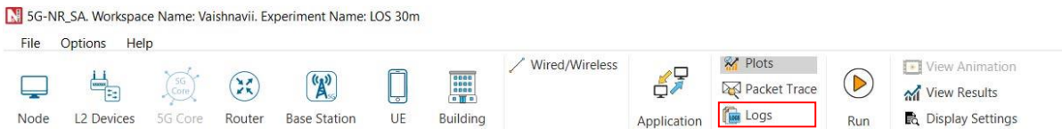
Figure 4-33: Enabling log files in NetSim GUI.
