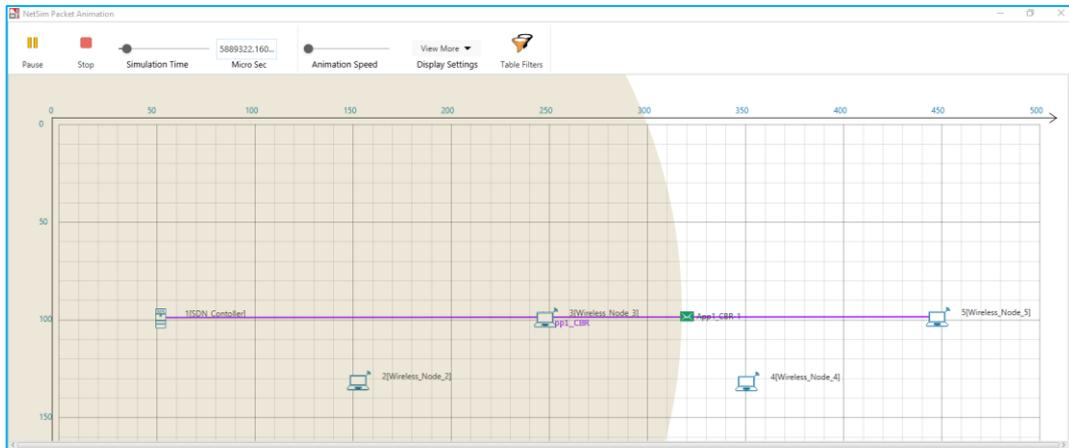
10. Configure static routes such that the packets will go through Wireless\_Node\_2 > Wireless\_Node\_4, to Wireless\_Node\_5.
